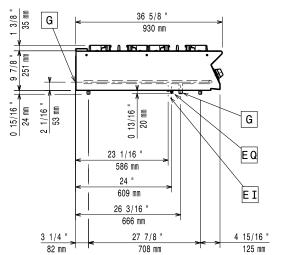
Electrical inlet (power) Gas connection
